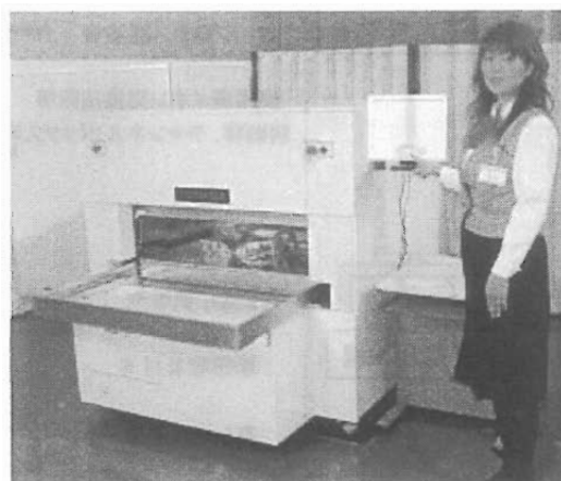
Fig.3 \beta/\gamma -ray Measuring System
