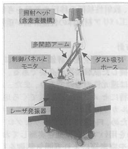
Fig.29 Laser Decontamination Equipment
